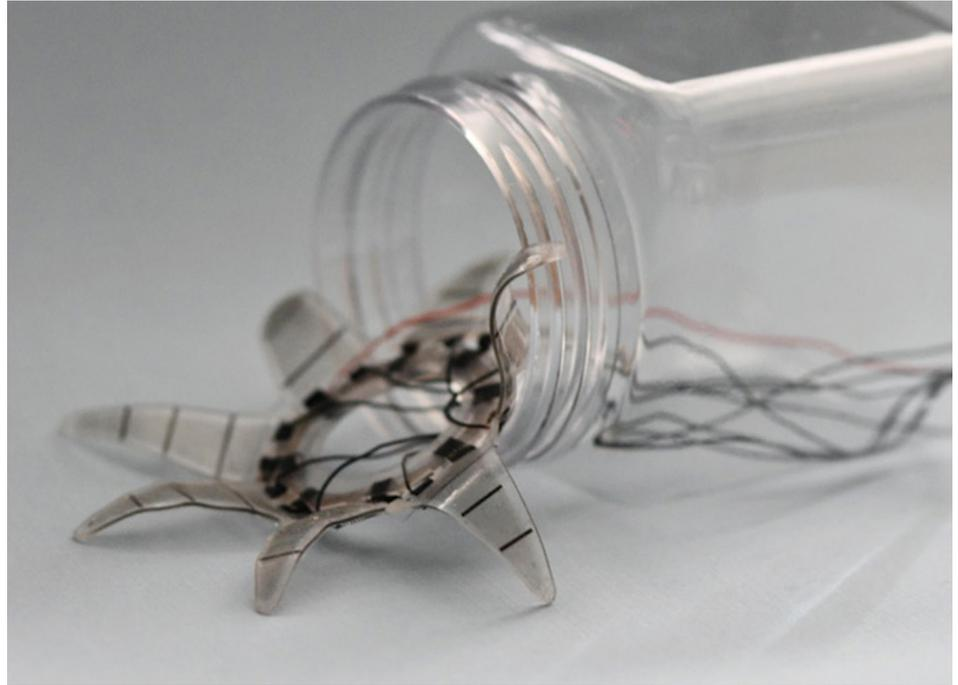
*Mihai Duduta, a researcher in the Faculty of Applied Science & Engineering, received JELF support for his team's work on soft robots, which can be made of a common polymer combined with carbon nanotubes (photo by Mihai Duduta)*
